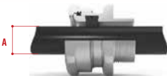
Cable gland with gasket with unarmoured cable
